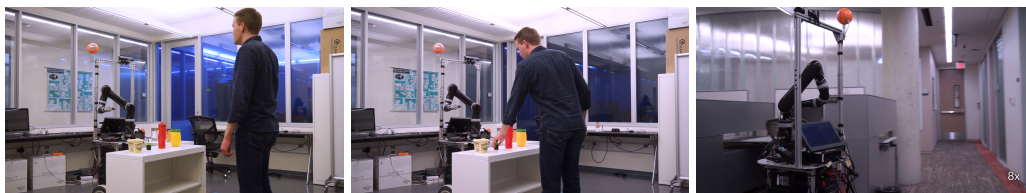
(a) The user gives the command verbally. (b) The robot learns the new rattling property. (c) The robot autonomously navigates to the target.
