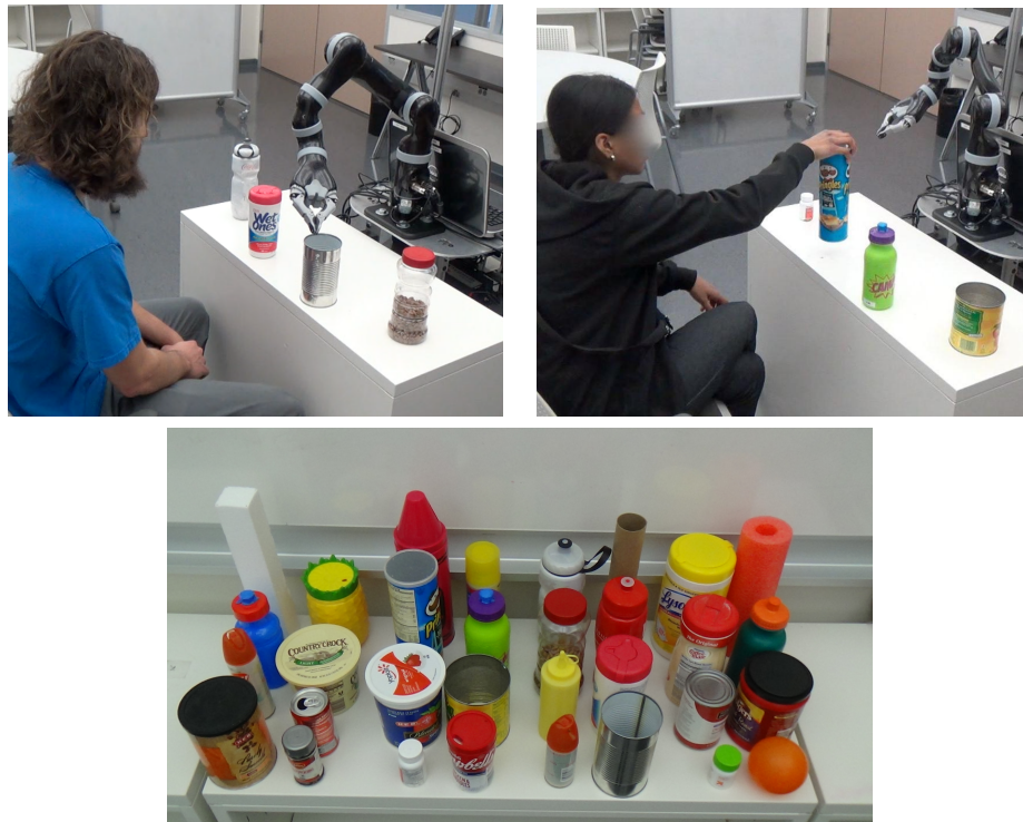
Figure 4.1: Top-Left: the robot guesses an object described by a human participant as silver, round, and empty . Top-Right: a human participant guesses an object described by the robot as light, tall, and tub . Bottom: objects used in the I Spy game divided into the four folds, from fold 0 on the left to fold 3 on the right.
