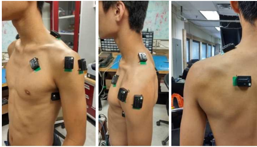
Figure 7.5: EMG sensors attached on a participant.
