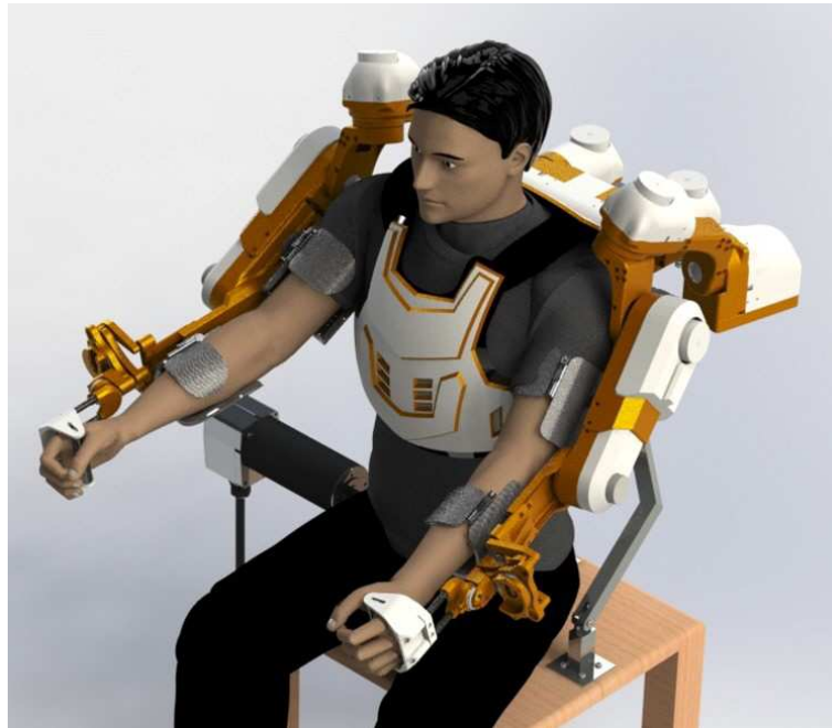
Figure 3.10: The CAD drawing of the upper body exoskeleton robot worn by a user ously with a C++ code that contains a high-level control by communicating via a shared memory interface.
