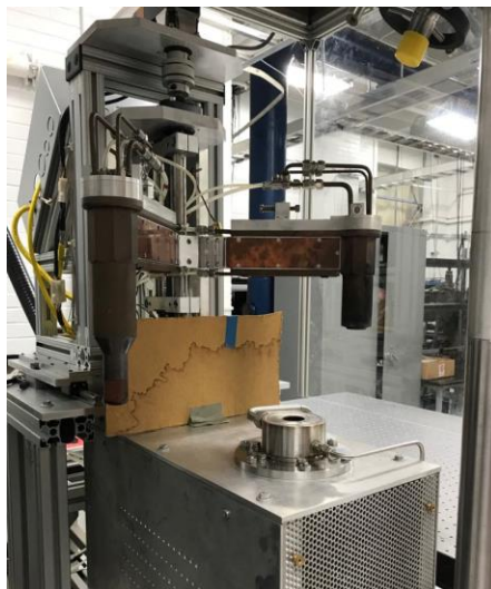
Figure 1.1: Photograph of the plasma torch facility. without plasma present.
