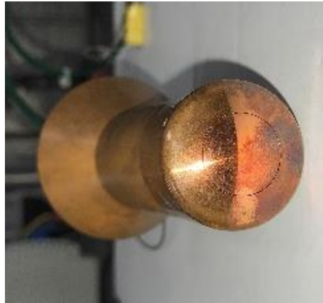
Figure 3.3: Photograph of the surface of the slug calorimeter.
