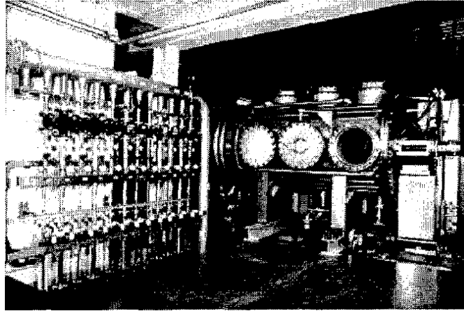
Figure 2.3: The 1.2 MW Plasmatron facility at the von Kármán Institute [3].
