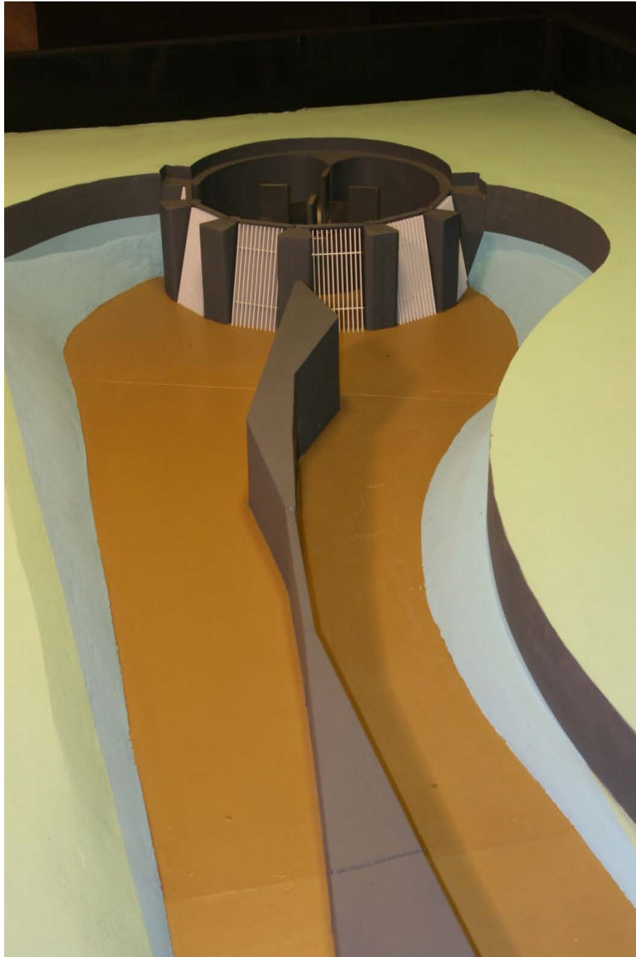
Figure 34: Waller Creek Tunnel Project; 1:33 Scale Model-Inlet Channelization
