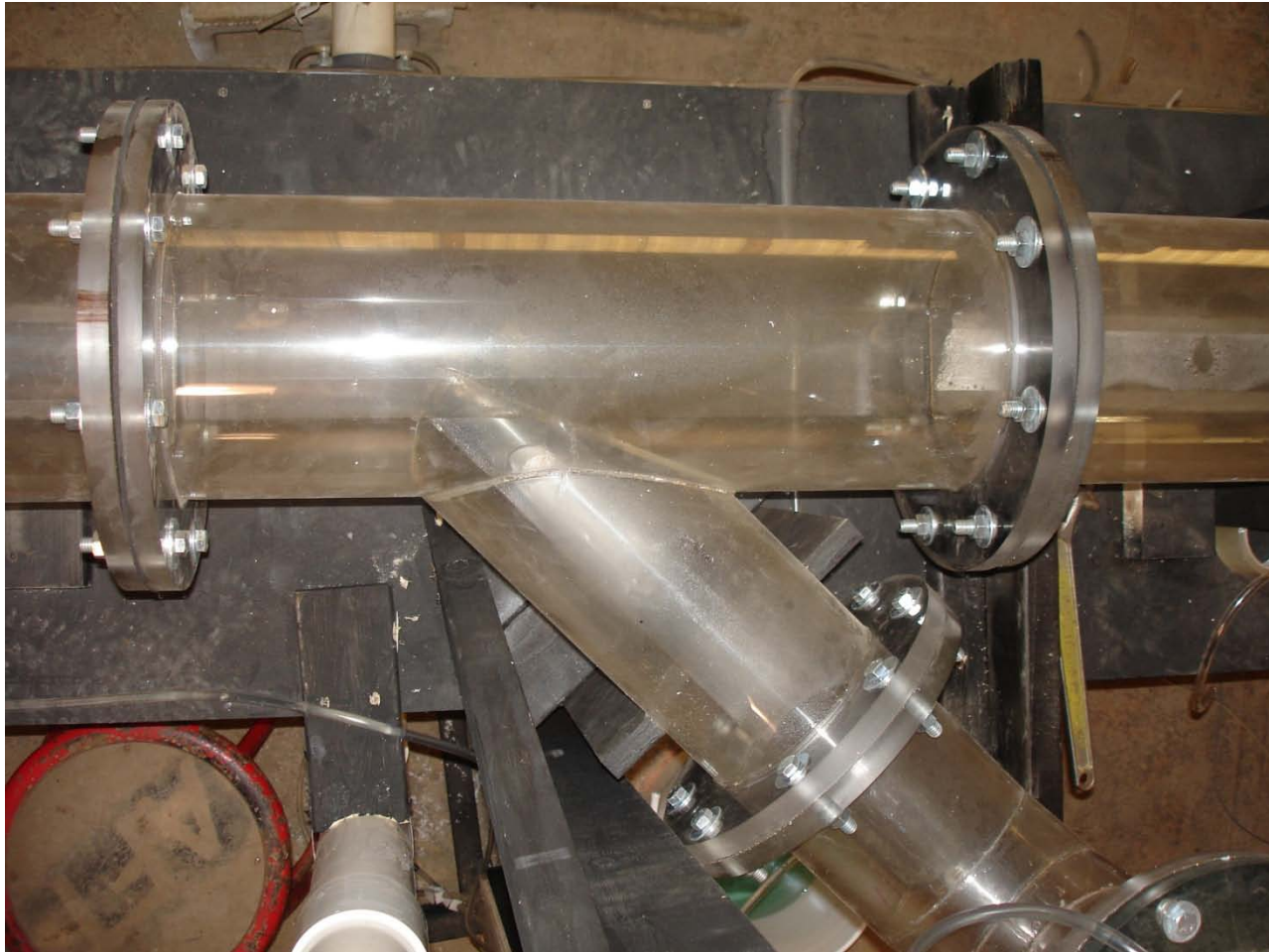
Figure 38: Waller Creek Tunnel Project; 1:33 Scale Model-8 th Street Lateral Junction
