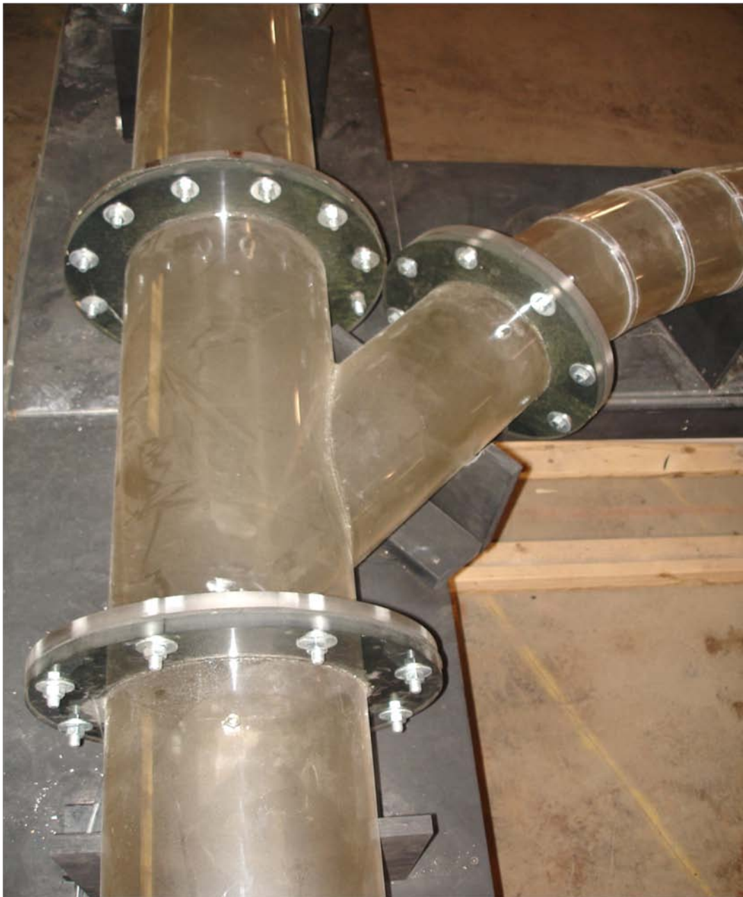
Figure 40: Waller Creek Tunnel Project; 1:33 Scale Model-4 th Street Lateral Junction
