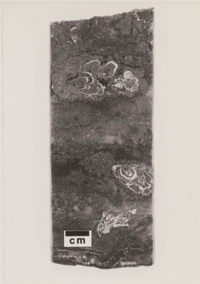
Fig. 4.10. Core photograph of massive sulfide section of anhydrite cap rock consisting of ramose Fe-sulfides interlaminated with tan chalky sphalerite; sample HB3-747.
