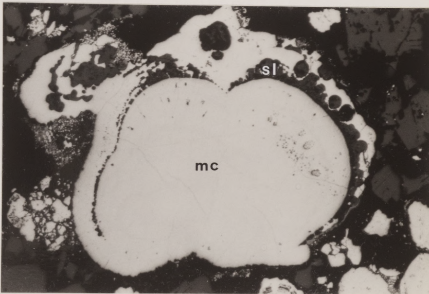
Fig. 4.15. Photomicrograph of colloform Fe-sulfide (mc) interlaminated and included with microcrystalline sphalerite (sl); sample HH2-878. Sphalerite bands and spheres were analyzed by microprobe, see text for discussion. Photo width is 2.5 mm; reflected light.
