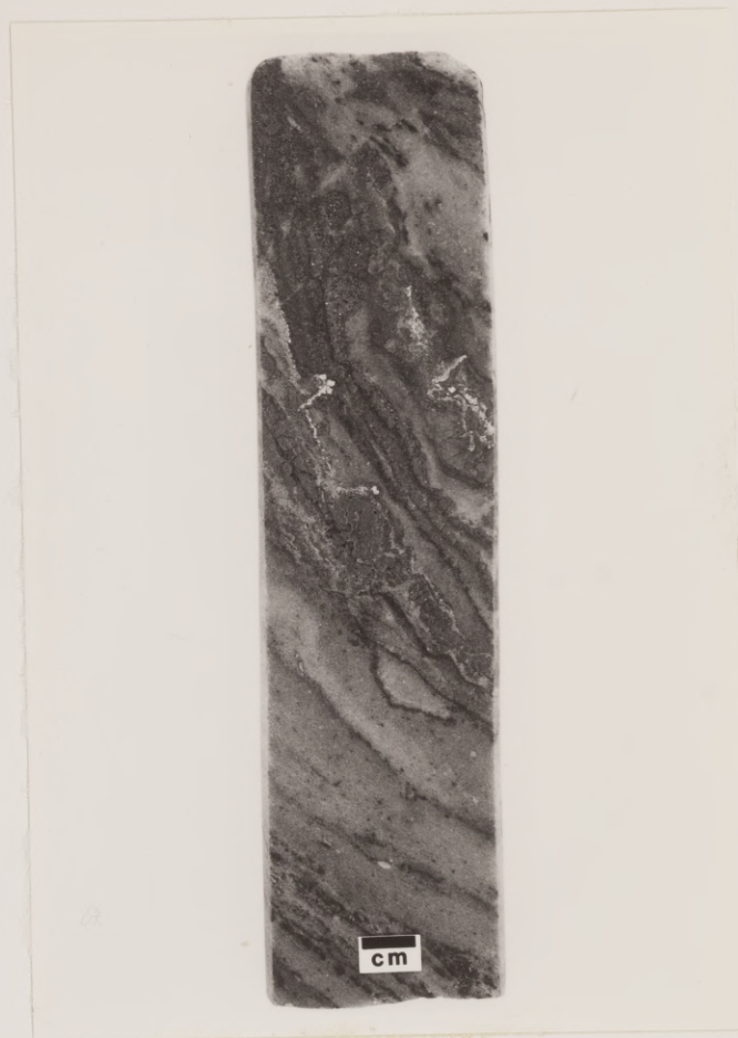
Fig. 4.5. Core photograph of steeply inclined sulfide laminae (roughly 45^\circ ) consisting of marcasite, pyrite, sphalerite and galena within anhydrite; sample HB3-934.
