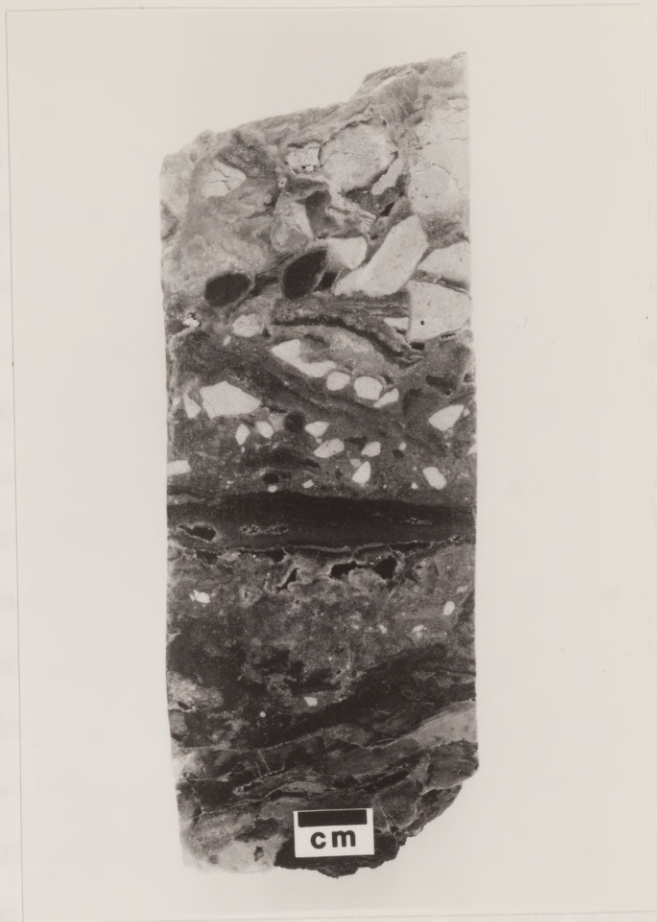
Fig. 3.23. Core photograph of angular sandstone inclusions in upper calcite cap rock; sample HB3-359.
