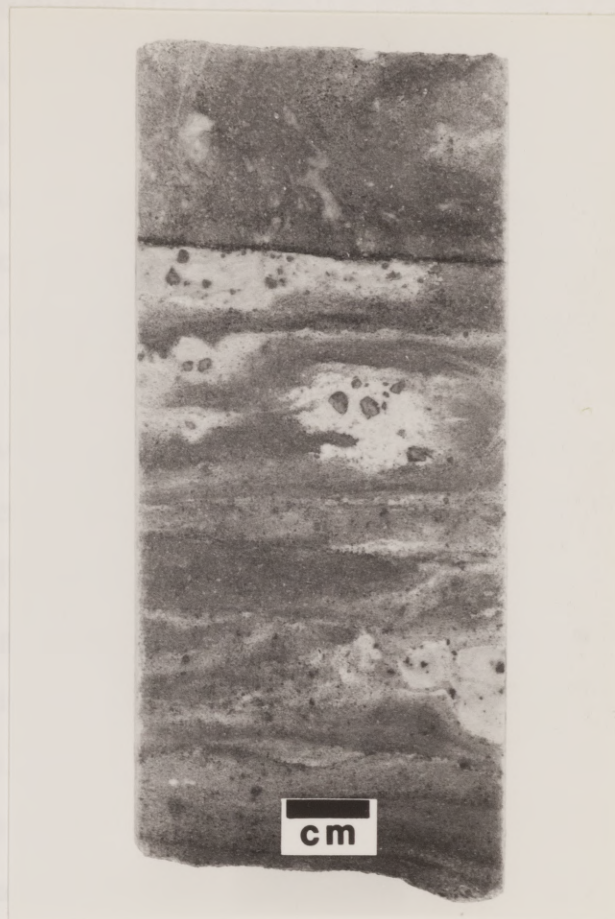
Fig. 3.21. Core photograph of sandy zones (white) in anhydrite cap rock; sample HH2-900. Clastic material also occurs as isolated dark rimmed clusters.
