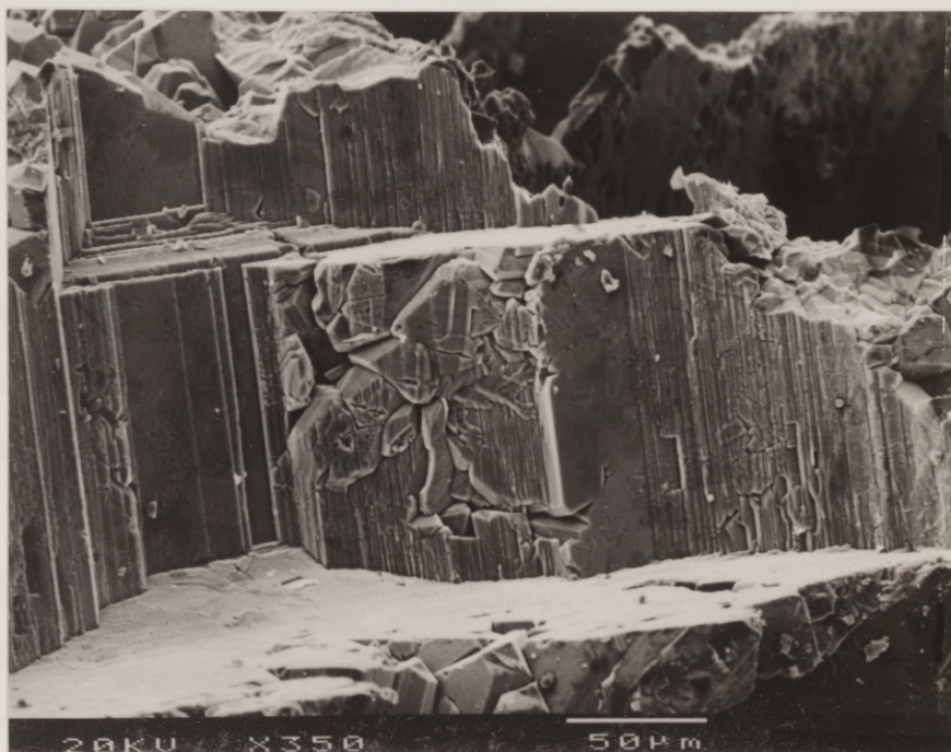
Fig. 4.6c. SEM photomicrograph of boxwork Fe-sulfide exhibiting geometric impressions left by anhydrite grain; sample HH2-404. Note sulfide surfaces show little corrosion. SEM photo width is 0.3 mm.
