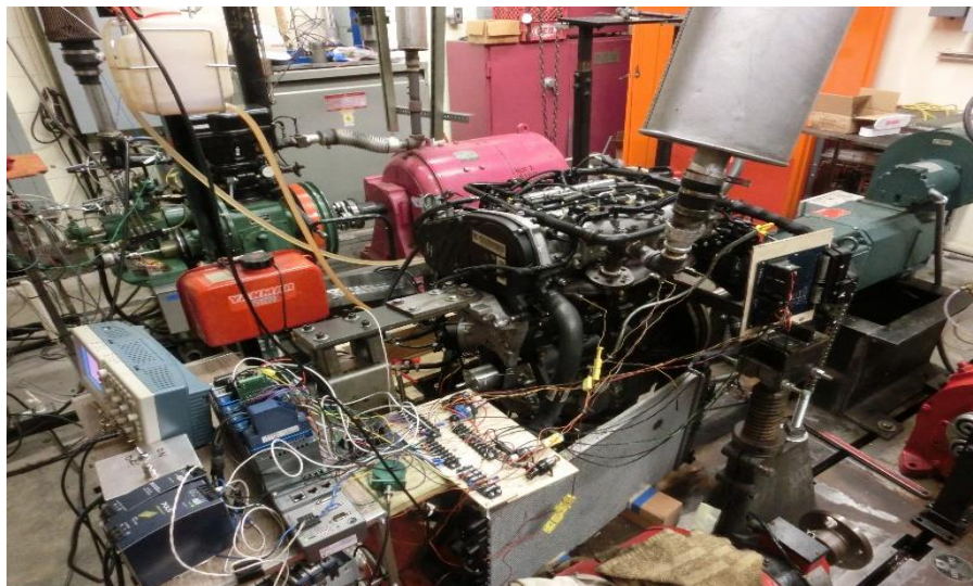
Figure 1-4 Engine, control hardware and data acquisition equipment
