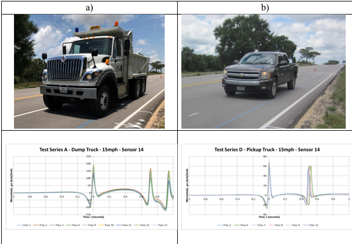
Figure 36: Example asphalt strain gages data recorded under controlled trafficking: a) heavy load (dump truck) trafficking; b) light load (pickup truck)
