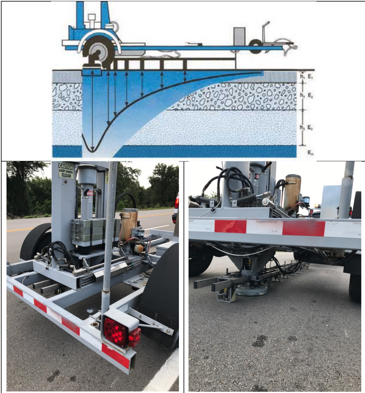
Figure 34: FWD equipment used during controlled testing campaign
