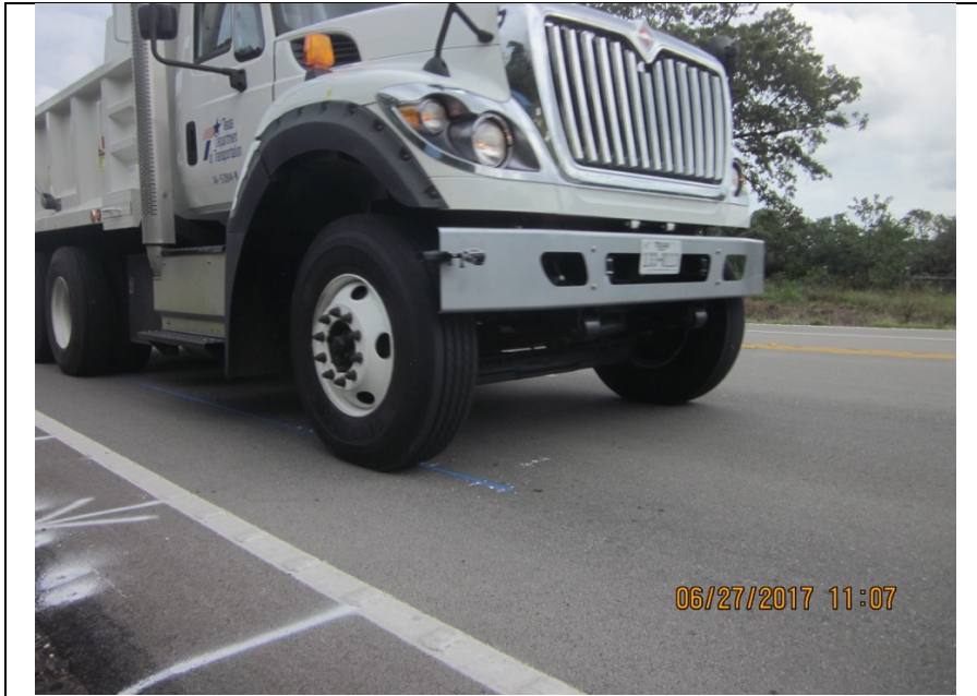
Figure 35: Maneuvering dump truck directly on the sensors during static testing
