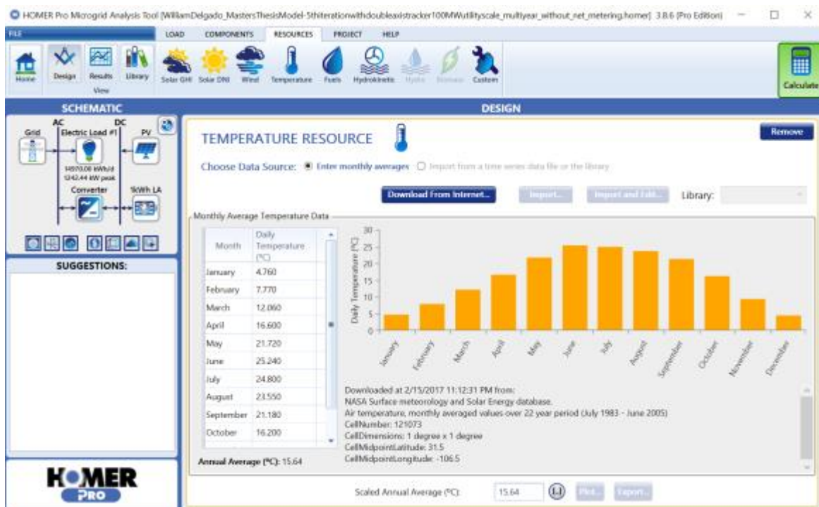
Figure 39 – Screenshot of project location’s average ambient daily temperature data downloaded from SMSED database
