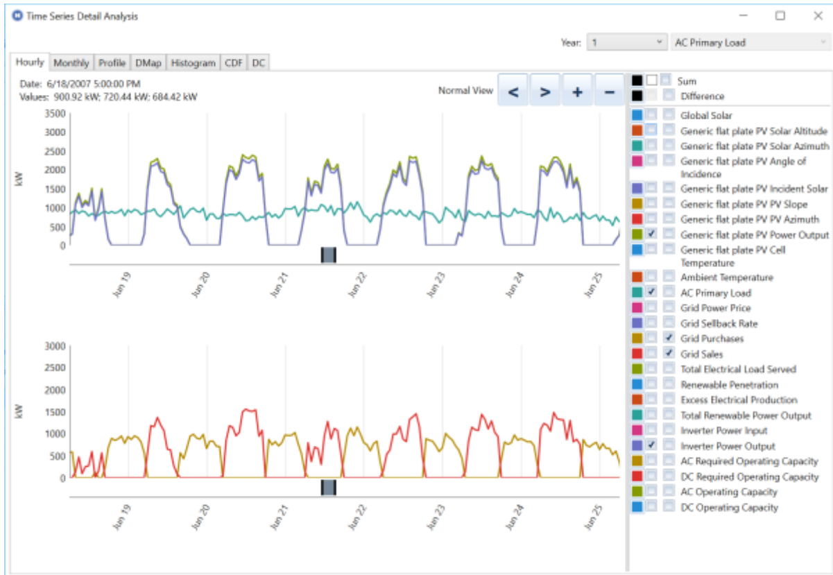
Figure 88 – Screenshot of time series plot that shows the predicted output values for various factors for each hour of each day of the year for the combination from Figure 87
