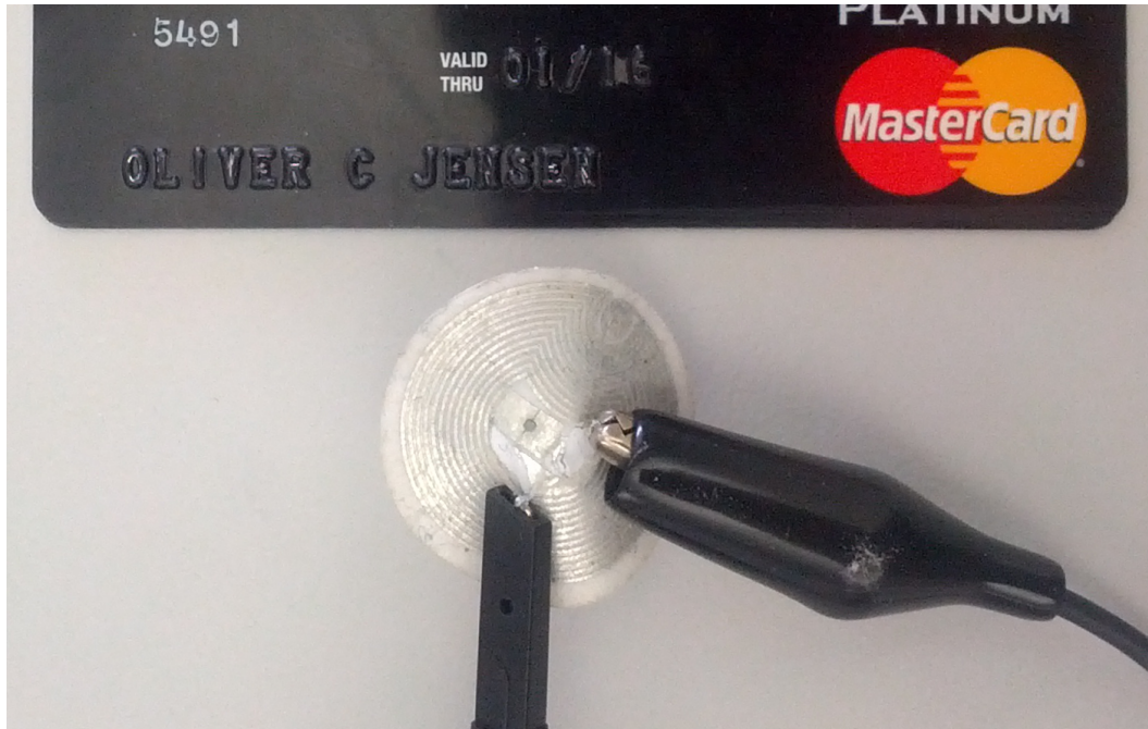
Figure 2.3: Eavesdropping Antenna (credit card for scale)
