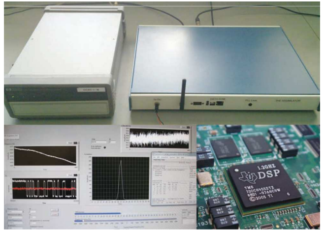
Fig. 4. Top: The prototype Assimilator device connected to a GPS time reference receiver. Lower left: Screen shot of a software GPS receiver tracking the Assimilator output and of the GPS time reference receiver's status page showing a timing lock. Lower right: The Assimilator's DSP core. This single chip performs all processing required for both signal tracking and signal generation.
