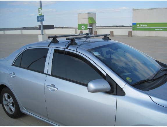
(a) The GPS and 2300 MHz antenna are placed on top of the vehicle.
