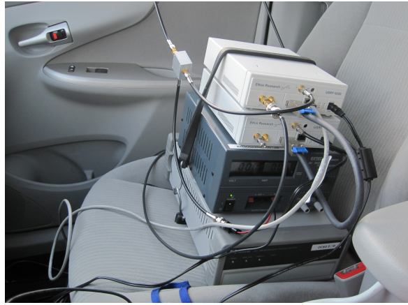
(b) The USRP N200 RF recording equipment, power supply, and OCOXO are placed inside the vehicle.
