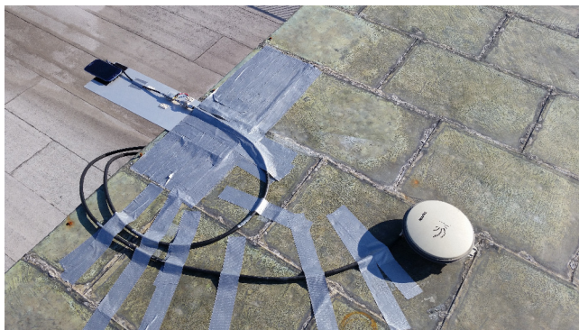
Fig. 15. Experimental setup for the Samsung Galaxy S3 antenna characterization study. The phone’s GNSS antenna and the survey-grade reference antenna, a NovAtel Pinwheel GPS-702L, are separated by approximately two meters.
