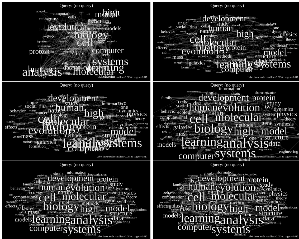
Figure F.1: Each phase of the layout algorithm is important for a compact though meaningful layout (via graph layout). The phases are (from left to right, top to bottom): random initialization, unconstrained simulated annealing, font scaling, feasible projection onto non-overlap set via reverse simulated annealing, constrained simulated annealing and finally a strong gravity phase of constrained simulated annealing. See subsection 12.5.1 for dataset description.
