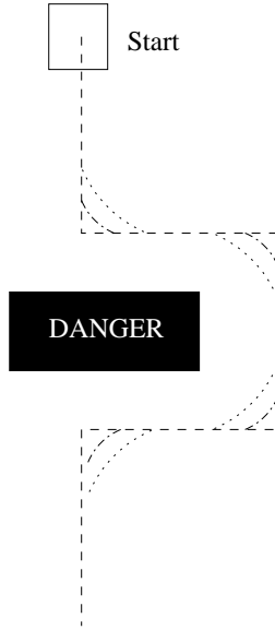
Figure 4.5: The approximate path along which the flock is influenced to travel. The dashed line shows the path if turns were instantaneous and the two arcs show the path when 100 or 200 time steps are used to turn. The flock starts in the square.
