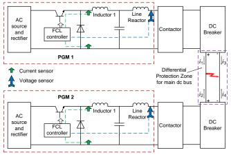
Fig. 3. Diagram of the converter FCL + differentional protection scheme.
