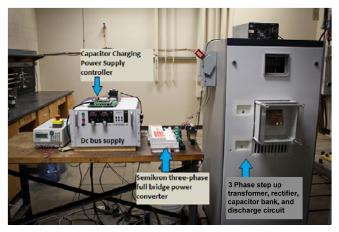
Fig. 10. Subscale CCPS set up with controller, dc bus, and capacitor bank.
