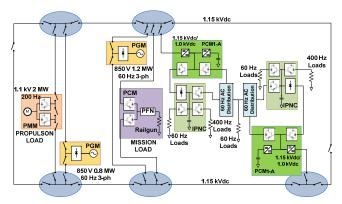
Fig. 1. Configuration of the UT-CEM dc microgrid test-bed.
