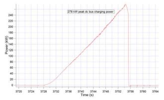
Fig. 12. Full-scale CCPS input power to charge capacitor banks.
