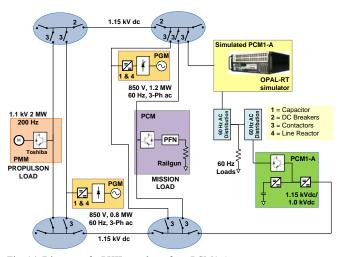
Fig. 14. Diagram of a PHIL emulator for a PCM1-A.
