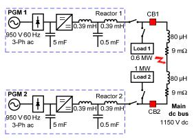
Fig. 4. SLD of the simulated system in Matlab/SIMULINK.
