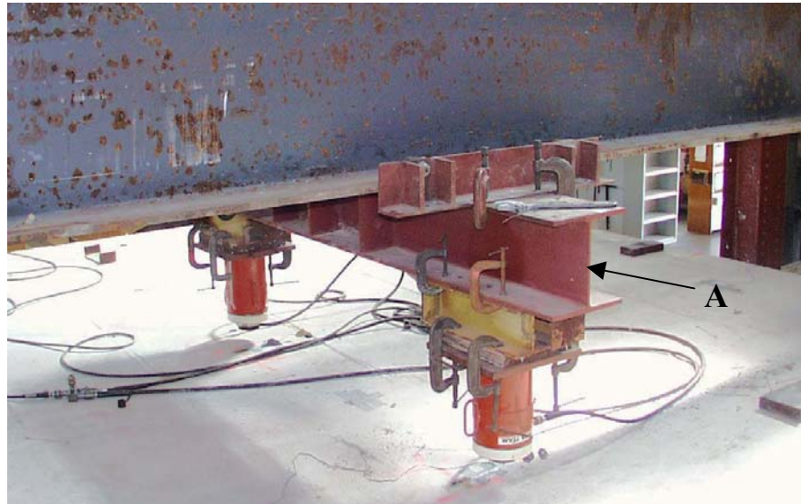
Figure 6.16 Attachment of actuators to load frame
