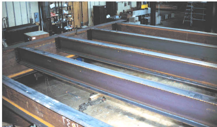
Figure 6.6 Transverse and longitudinal steel beams in laboratory model
