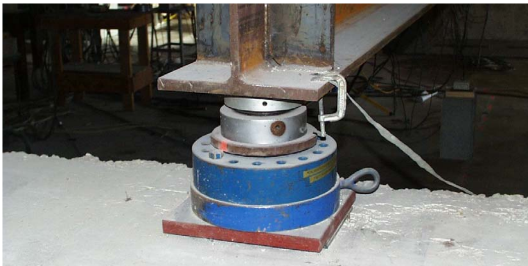
Figure 6.4 Transverse beam placed on (top to bottom) a swivel plate, a load cell, and leveling plates
