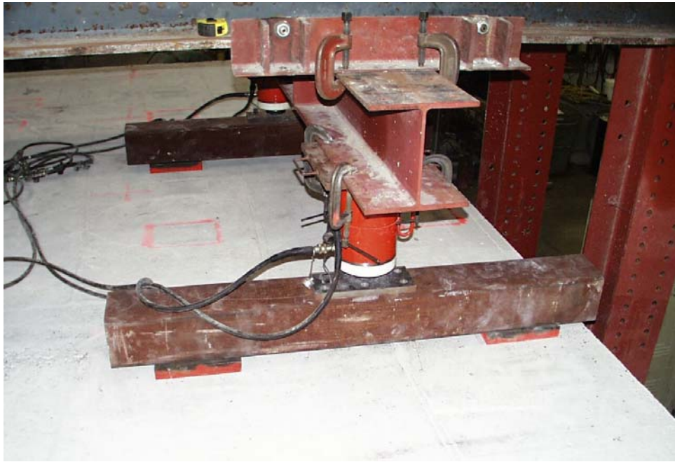
Figure 6.18 Approximation of tandem axle with structural tubing and rubber pads
