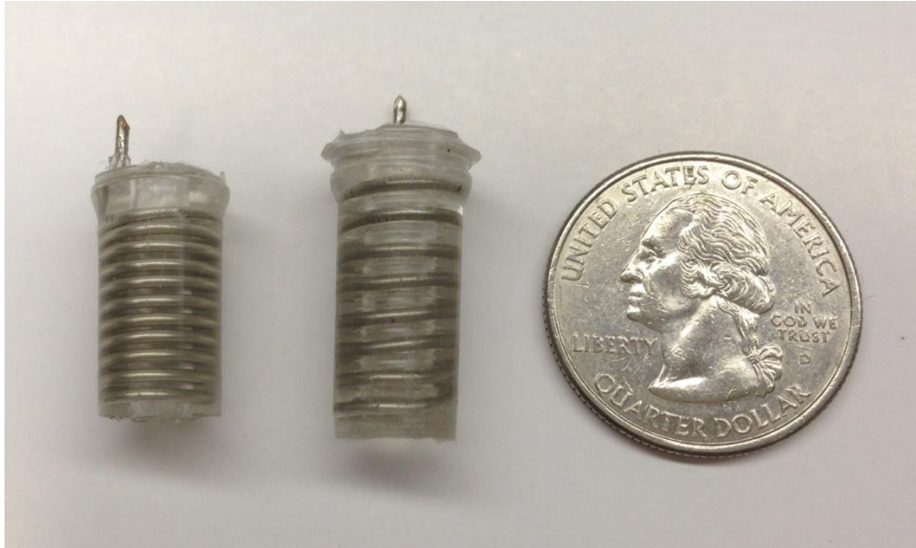
Figure 3.6: The manufactured antenna sensors with PDMS packaging.
