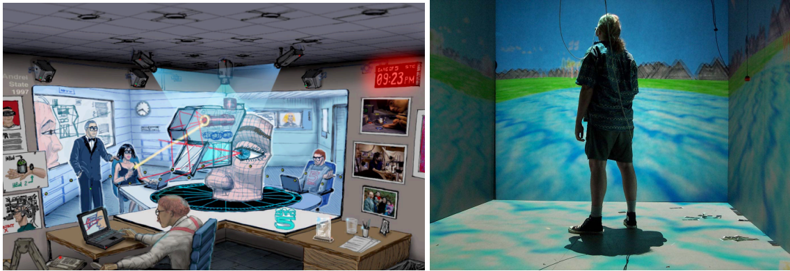
Figure 36: Left: Conceptual sketch for the Office of the Future (1998); Right: The CAVE virtual environment with rear projection screens
