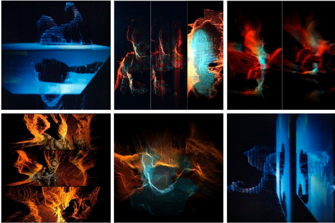
Figure 73: Screenshots of real-time 3D point cloud volumetric renders using our system with openFrameworks and Xbox Kinect v1 (overlay of the pixel-based RGB image with 3D point cloud).
