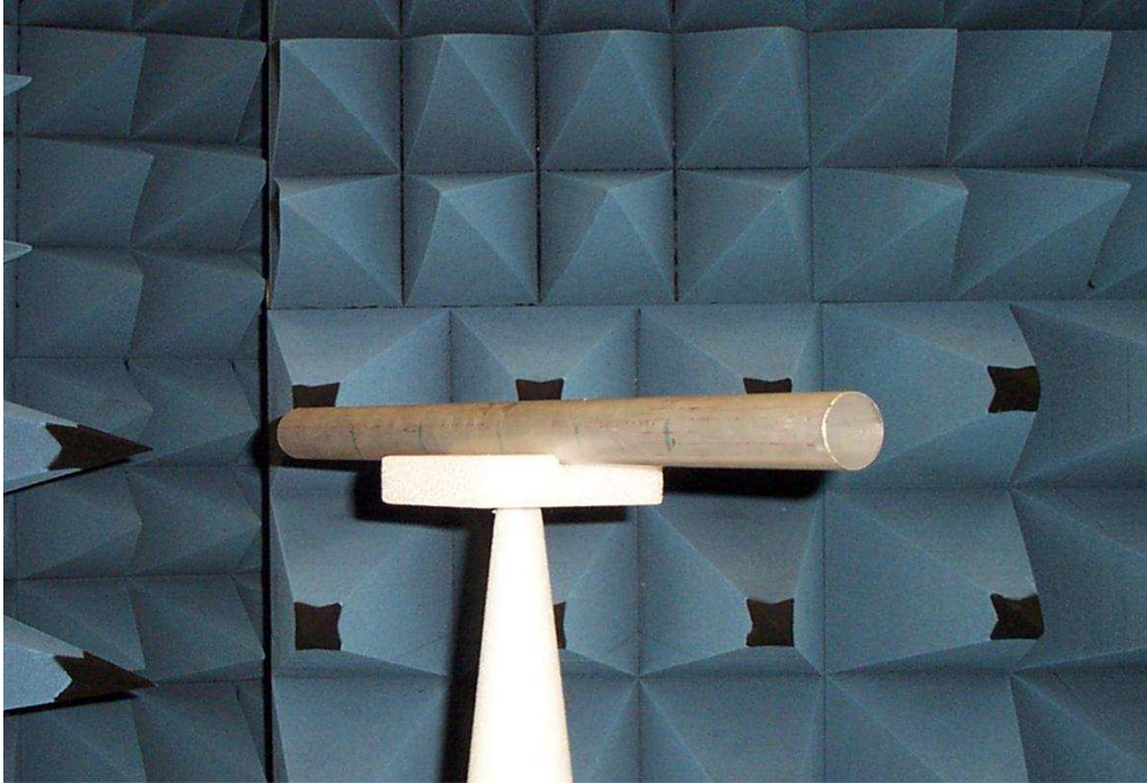
Figure 12 Circular cylinder used for measurement of the open-ended duct and the duct with two open ends
