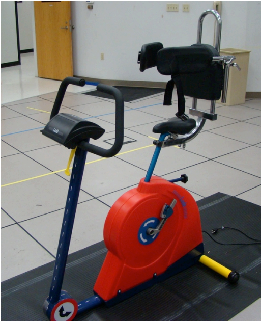
Figure 3.1: Ergometer with trunk support that was used during this study.
