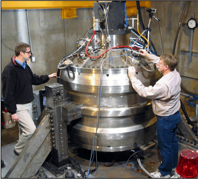
Figure 3. 100 kW-hr, 2MW flywheel in testing
