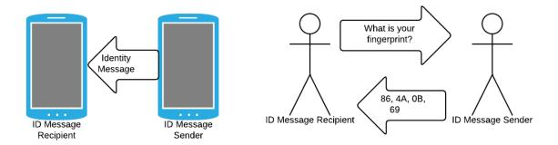
Figure 5.2 – Identity Exchange, Manual Authentication
