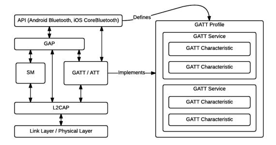
Figure 2.1 – Bluetooth Low Energy Protocol Layers
