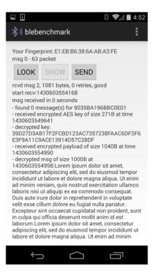
Figure 5.5 - Receipt and Decryption of AES Key and Original Message
