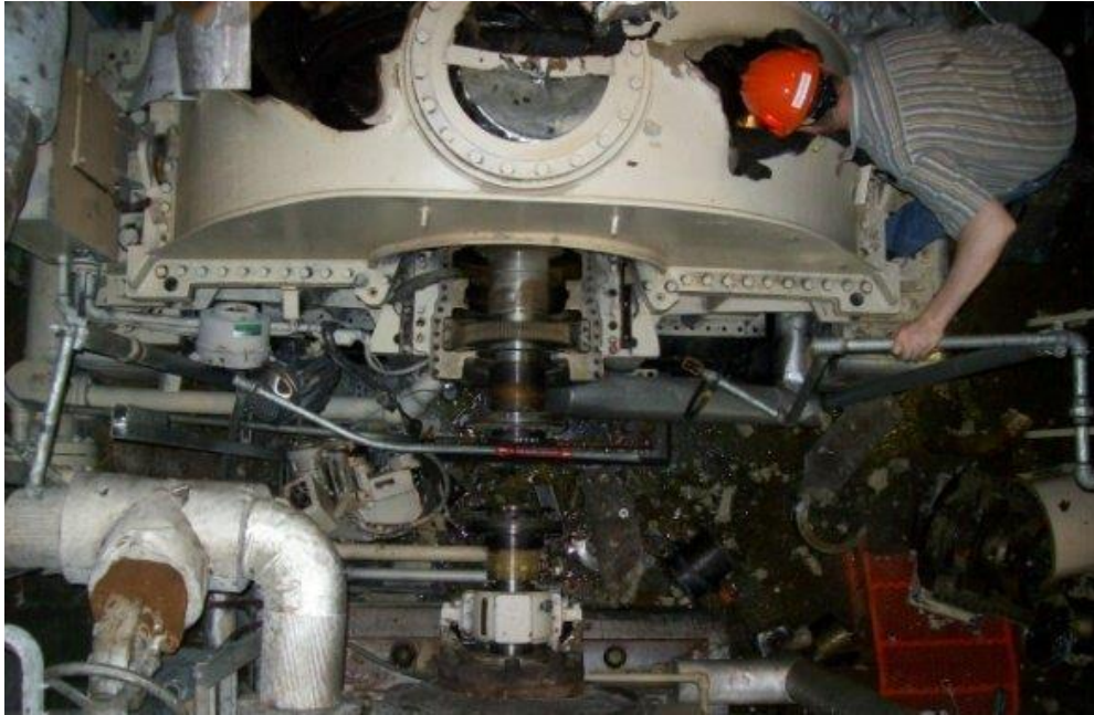
Figure D-1: Wreckage on the exhaust hood and low-pressure end bearing
