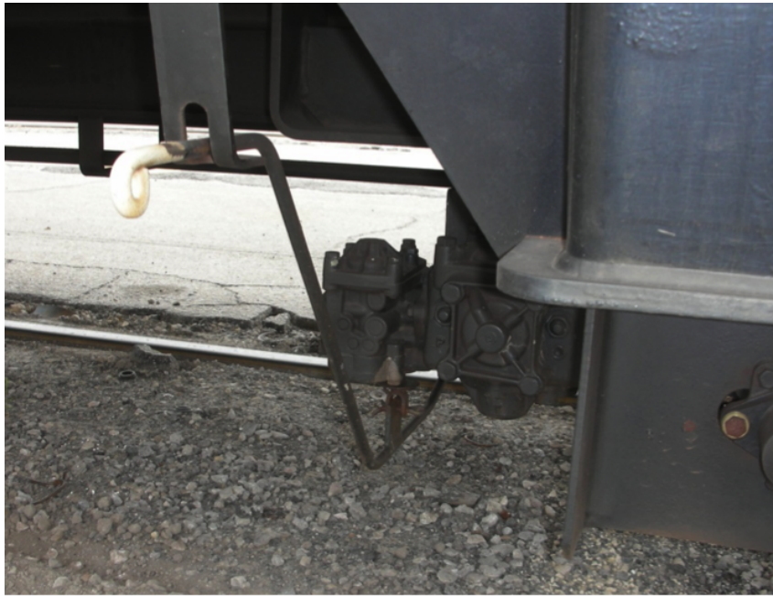
Figure 11.8: Lower position valve with no direct obstructions
