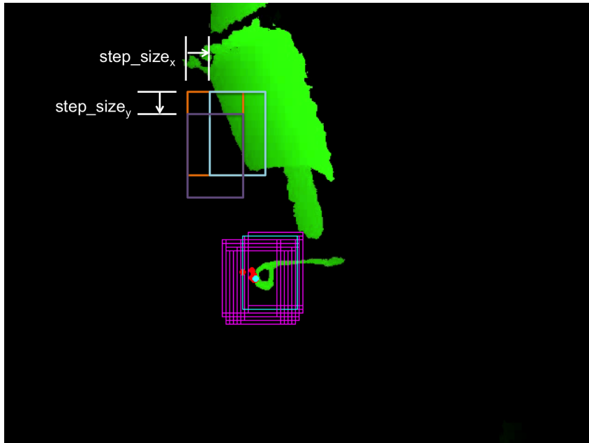
Figure 7.2: Window step-size schematic (for clarity, the labeled step is much larger than the actual step size, which gives the spacing between the “true positive detections”)
