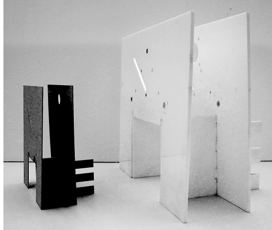
Figure 4.4: Use of scaling in design of a fluid flow chamber: (left) scaled model, and (right) full size model. Use of a scaled model saved time and material during tests of system interfaces.
