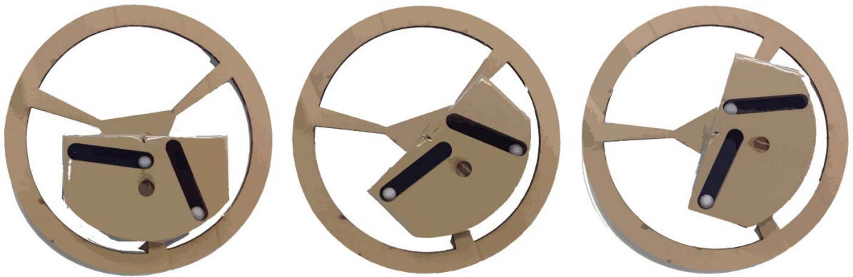
Figure 2.5: An example isolated subsystem prototype. This is a testing rig for a three-phase mechanical pitch sensor on a rolling cart robot. The system is completely isolated. Electrical contacts are not included. The only function being tested is the relationship between tilt angle and the position of the rolling contacts. The basic phenomena of the sensor geometry can be evaluated without time expenditure on the wiring or other systems.
