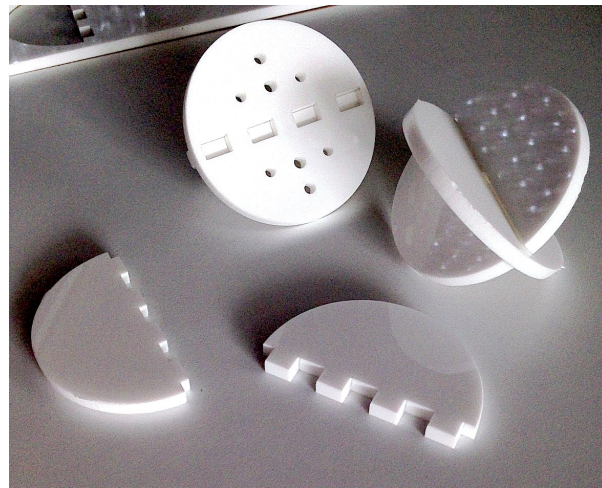
Figure 4.5: Use of subsystem isolation in design of a joint. Several joint concepts are pictured. These isolated prototypes were significantly easier to test without encumbrance of the full system.
