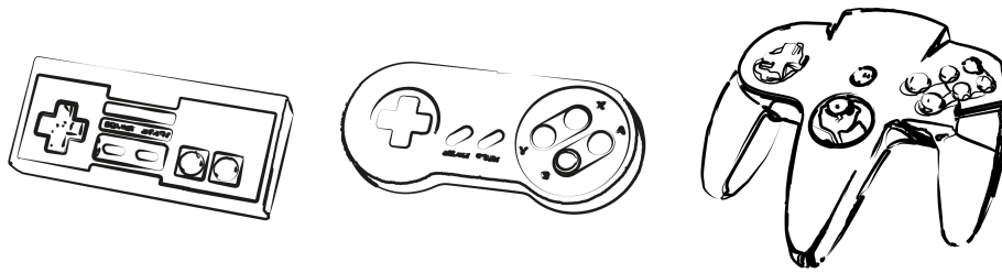
Figure 2.8: An example of iterative design. These three controllers show vast improvements in ergonomics with each iteration.
