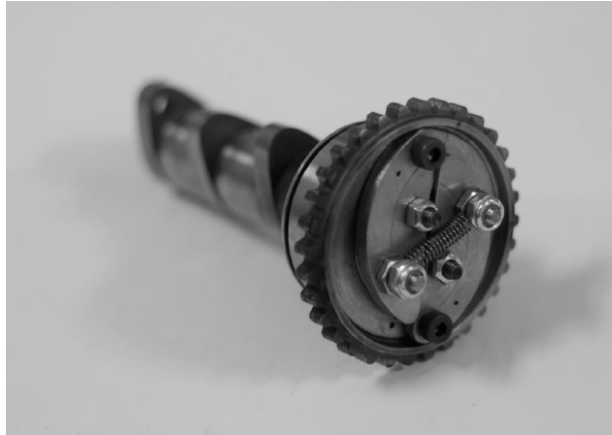
Figure 4.15: An example prototype from the capstone design study, a cam phaser.
