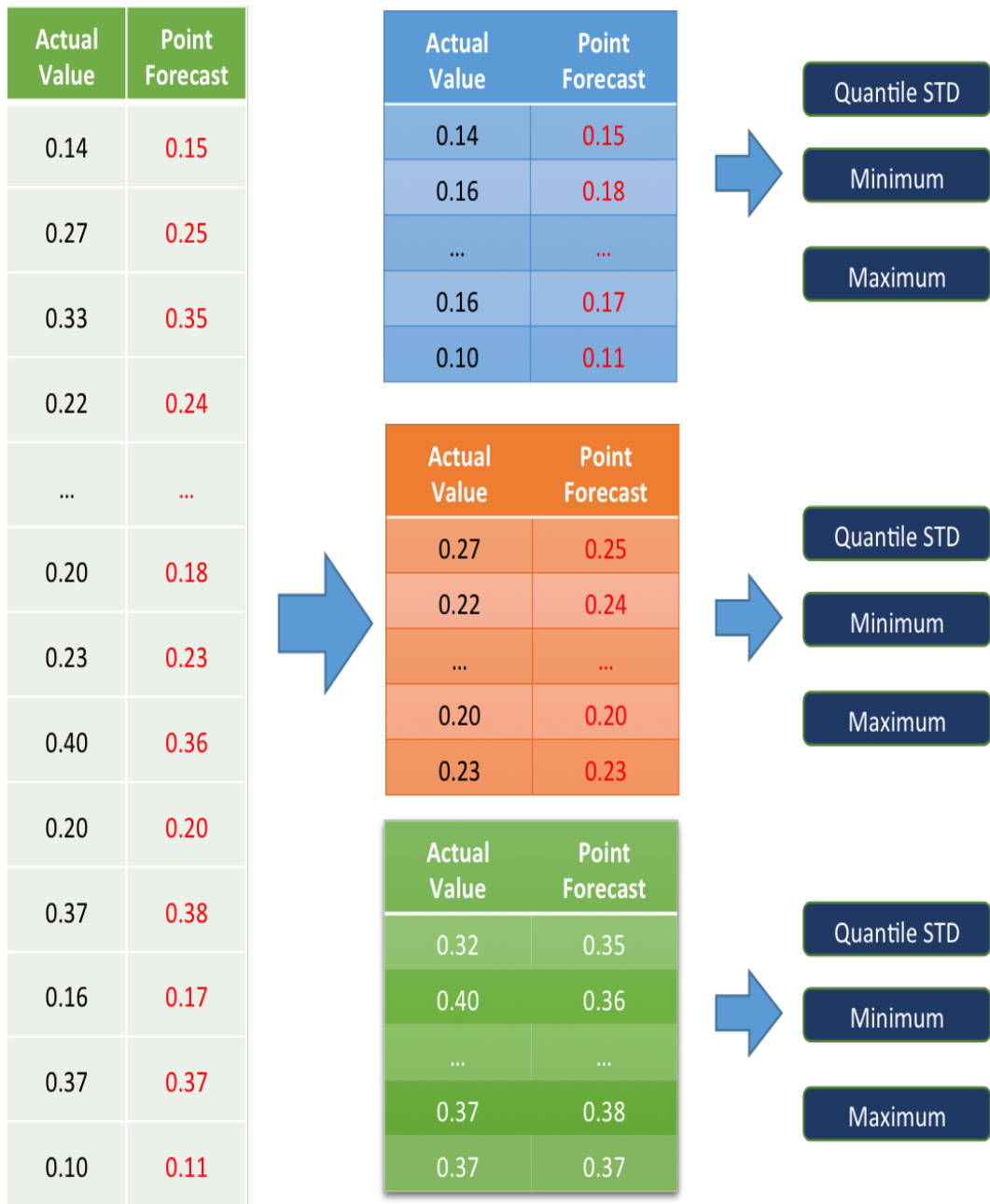
Figure 2.10: The point forecasts are clustered into ten clusters with respect to their power levels.
