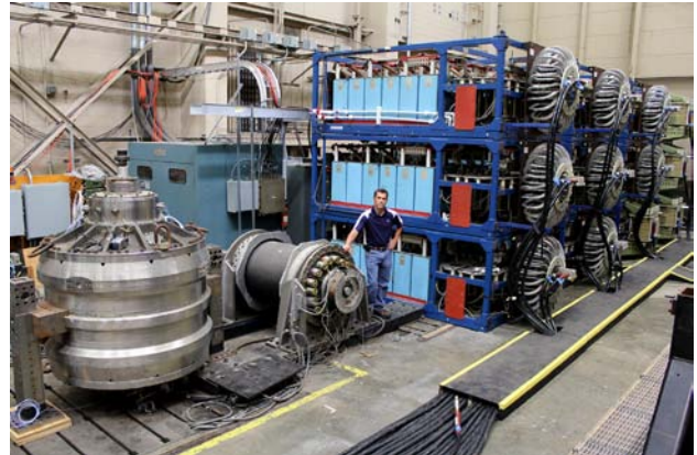
Figure 2: Embodiments of three different storage technologies. From left to right are a flywheel, a pulsed alternator, and a capacitor bank. The flywheels stores 480 MJ, The pulsed alternator stores 22 MJ. The capacitor bank stores 12 MJ.
