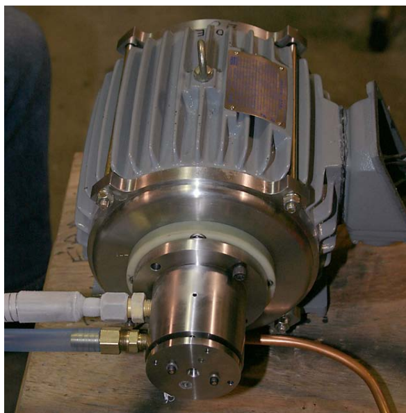
Figure 11. High temperature superconductor motor using bulk trapped field magnet.
