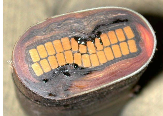
Figure 4. Coil removed from 155°C oven
