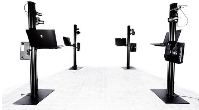
Figure 2.5: A structured light based body scanner from 4DDynamics with four Mephisto EX scanner units. Each units consists of an HDTV machine vision camera as the main geometry camera, a digital projector, and a Canon DSLR texture camera.
