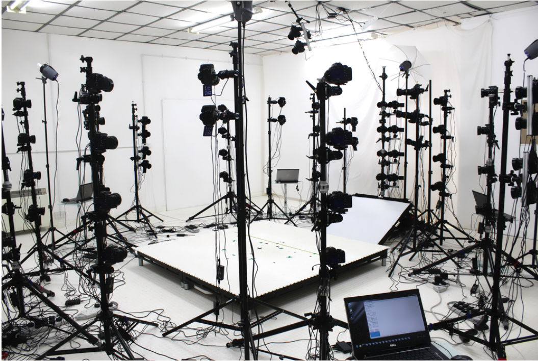
Figure 2.6: The stereo vision 3D imaging system deployed by Infinite-Realities (UK). System consists of 115 Canon DSLR cameras and studio lighting equipment.
