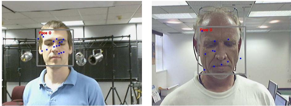
Figure 5.2: Examples of face detection using the Haar-like face detector and SIFT feature extraction. The gray rectangles indicate the detected face regions, while the locations of SIFT keypoint are denoted as blue dots. The number and the positions of SIFT keypoints may vary across images of the same person.
