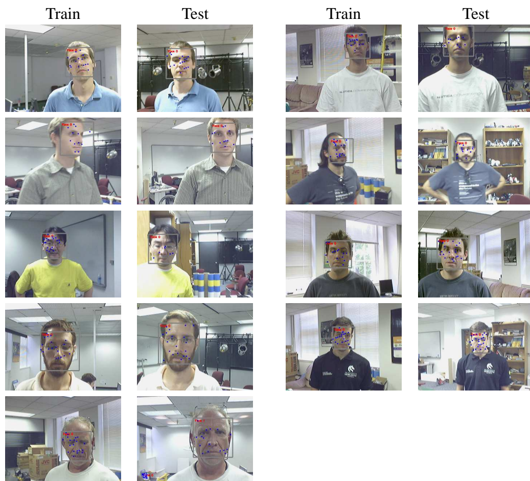
Figure 5.8: Sample images of the UT Austin Villa facial video database showing the detected face regions as gray rectangles and SIFT keypoints as blue dots. The Haar-like face detector scans for face regions in each frame. Each of the detected face regions is converted into grayscale and resized to 24 \times 24 to extract SIFT keypoints. On average, each face contains about 10 \sim 20 SIFT keypoints.
