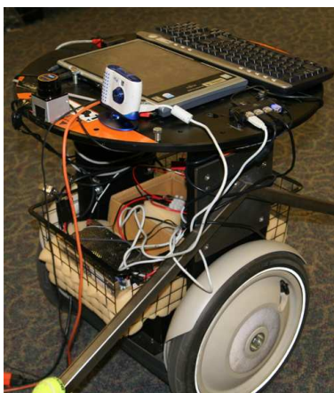
Figure 5.1: The UT Austin Villa facial video database is constructed using the mobile robot shown in this figure. It consists of a Segway RMP, a webcam, a URG-04LX laser rangefinder, and a laptop. Analyzing the input images from the webcam and the distance information from the URG-04LX laser rangefinder, appropriate motion commands are sent to the Segway RMP to turn and to move forward and backwards.
