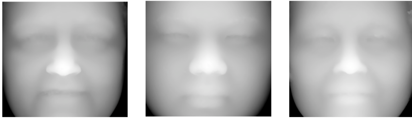
Figure 4.9: The sub-regions of the facial range images that were employed for the eigensurfaces and fishersurfaces 3D face recognition algorithms.
