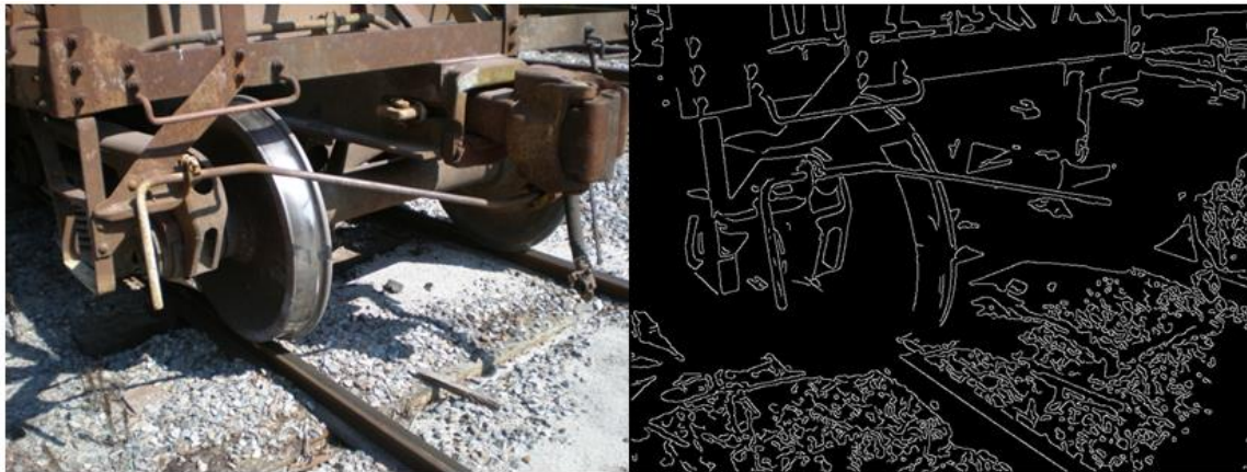
Figure 5-4: Original image (left) & detected edges using Canny (right)
