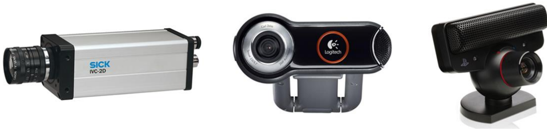
Figure 4-3: Digital 2D cameras a) SICK smart camera [SICK, 2006], b) Logitech Pro 9000 webcam [Logitech, 2013], & c) PlayStation Eye [Sony, 2013]
