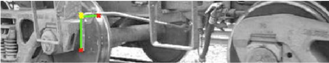
Figure 5-9: Uncoupling lever assembly detection – geometric fitting
