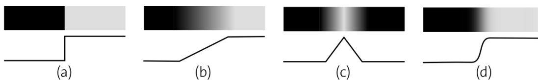
Figure 3-4: Edges types (a) step, (b) ramp, (c) roof, and (d) smooth [Cattin, 2012]
