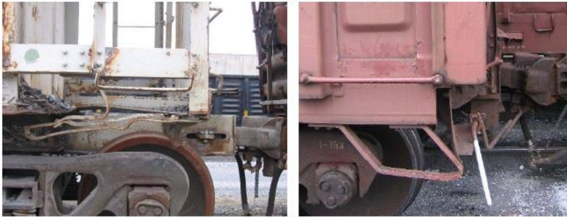
Figure 2-1: Extreme deformation to sill steps on rolling stock [Edwards, 2006]
