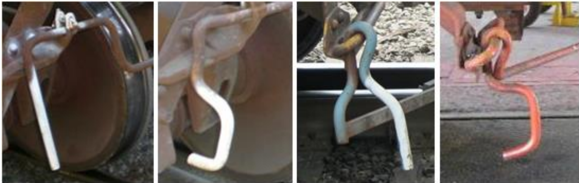
Figure 5-2: Uncoupling lever handle types
