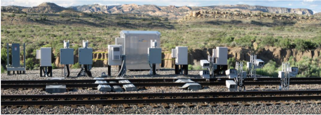
Figure 2-2: Beena Vision wayside inspection system [Nayebi et al., 2012]
