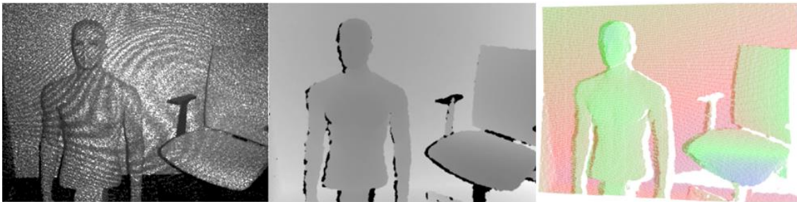
Figure 4-12: (Left to Right) a) IR image of scene, b) Grayscale distance image, & c) Color coded point cloud [Metrilus, 2013]
