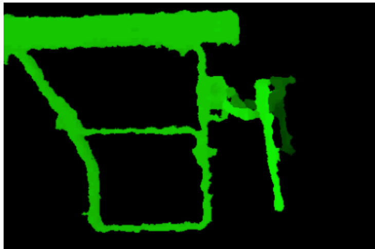
Figure 5-18: Filtered depth map (pixels shown are 0 to 1.5 m from camera)
