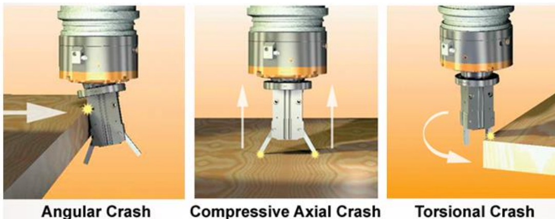
Figure 4-17: Collision sensor response modes [ATI-1, 2013]
