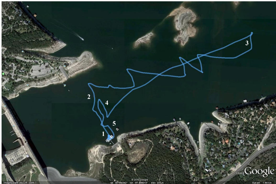
Figure 2.10: GPS map of typical transmitter path during experiment. Various transmit positions are enumerated where the mobile boat communicates back with the array mounted to the barge located at position 1.
