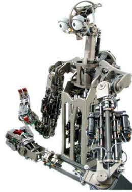
Figure 2.3: Two ball screw SEA designs from the Massachusetts Institute of Technology. a) The Spring Flamingo SEA and b) The Domo Humanoid SEA (Edsinger-Gonzales and Weber, 2004).
