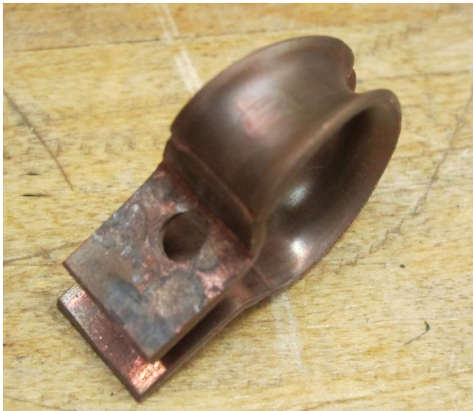
Figure 6.5 A bowed coil from a megagauss low-current shot on a 1/8th inch thick solid coil. This coil behavior agrees well with simulations and experiments done at other facilities as depicted in figure 6.5.
