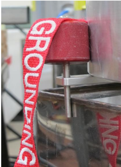
Figure 4.9 The red pins used to hold and retract the grounding levers. The warning strap is labeled “grounding lever retracted”. These pins must be in place for the capacitors to be charged.
