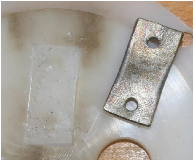
Figure 5.1 A steel shorting bar after the first megaamp shot on the full megagauss system. Magnetic pressure launched the bar vertically, causing it to collide with the debris shield plate above it. The shorting bar itself displayed signs of pinching and heating effects.
