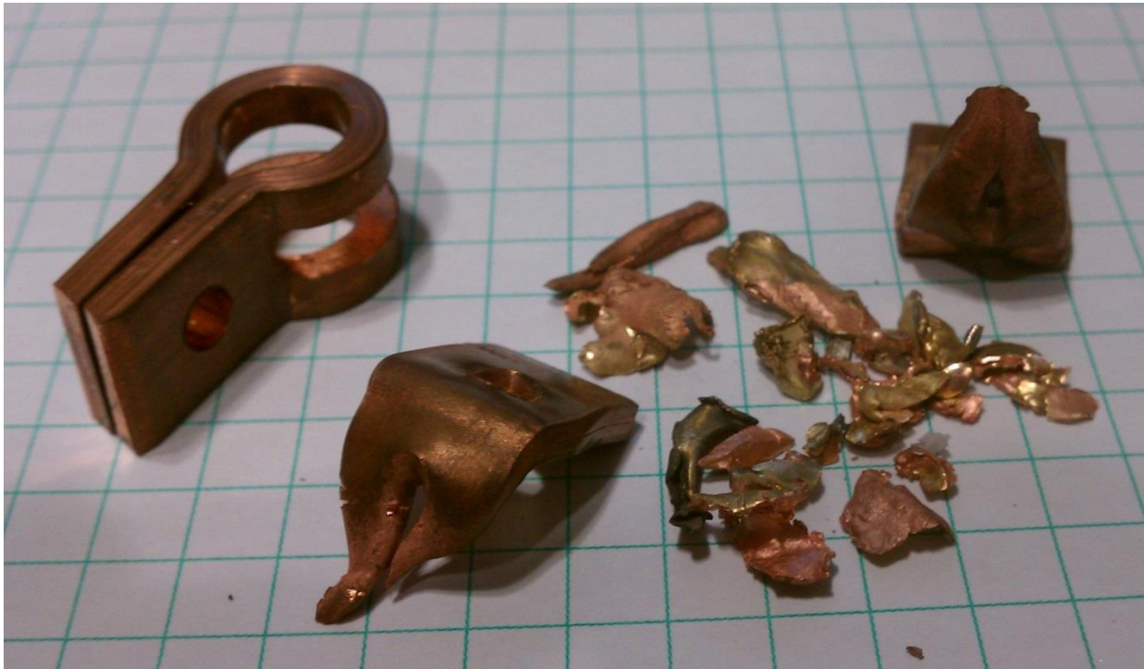
Figure 5.5 An image of the coil fragments from vacuum shot 13. To the left is an identical coil prior to being shot. Many of the copper fragments had to be extracted from the aluminum wall of the chamber where they were buried from impact.
