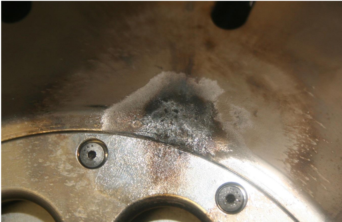
Figure 5.4 The results of an arc in atmosphere on the stainless steel transmission line anode plate. Panchen breakdowns in atmosphere concentrate all the current in a single arc and are particularly catastrophic.
