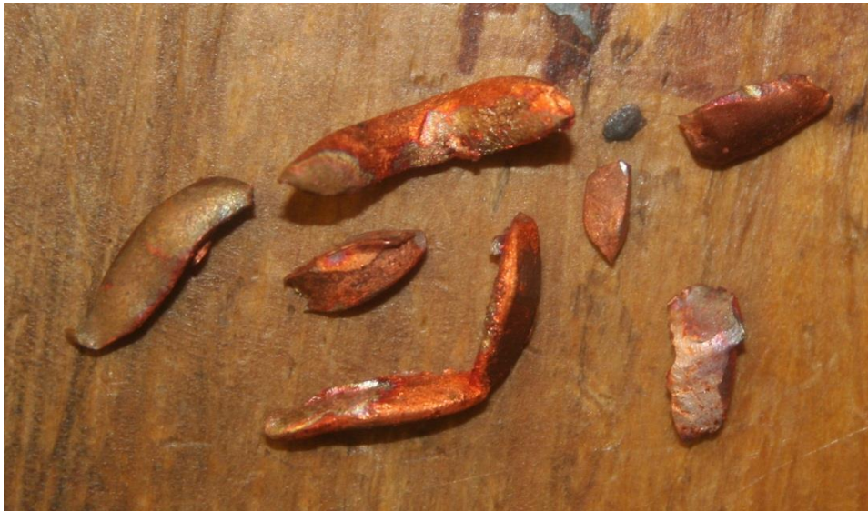
Figure 6.3 This image shows fragments from a slotted coil that fragmented into pieces several millimeters in length. The ends of these fragments are often sharp from current concentration.
