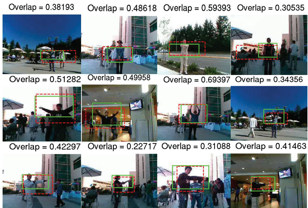
Figure 4.6: Detections for Clapping (top row), Waving (middle), and Boxing (bottom) from MSR Actions. The bounding boxes of our detections (red) align closely with those of the ground truth (green), after only 15 rounds of annotation.
