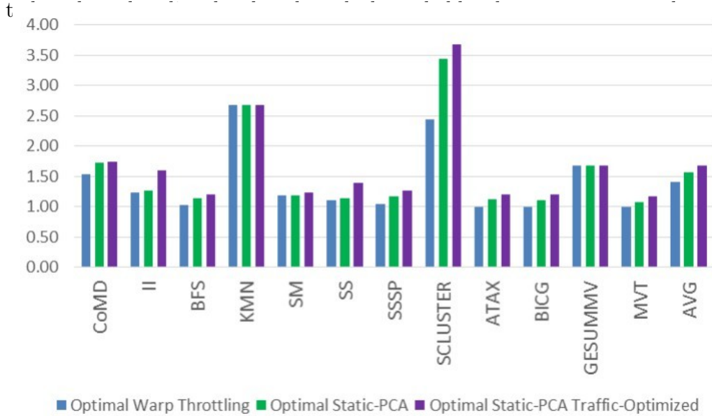
Figure 4.23: Comparing the speedup of optimal warp level throttling, optimal static PCAL and static PCAL with with NoC traffic optimization (Static PCAL-BTO).(Normalized to baseline which allows max warp/SM)
