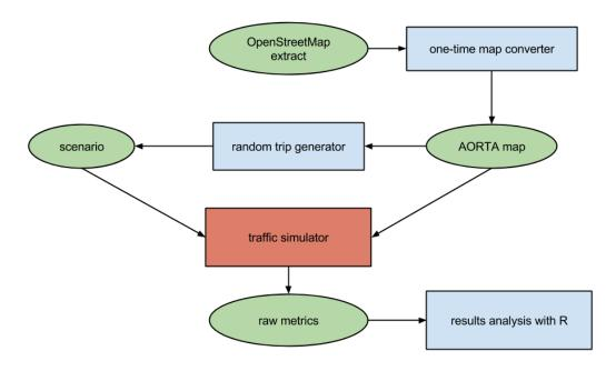
Figure 5: The interaction of the traffic simulator with other components
