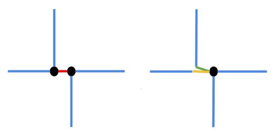
Figure 2: A short road (left) and its removal (right)
