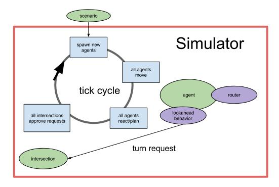
Figure 6: The main loop of the AORTA simulator
