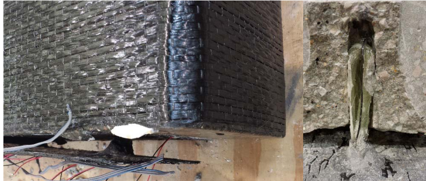
e) Pull-out of GFRP anchor
