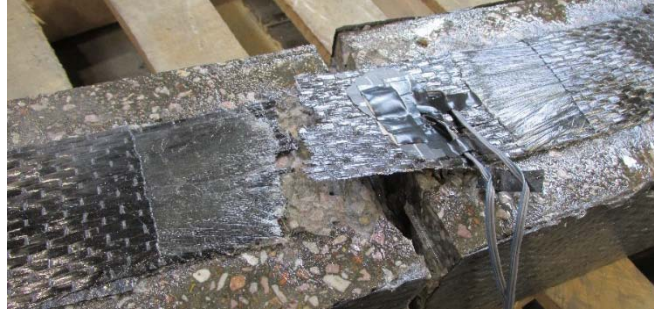
Figure 4.2 Specimen with CFRP rupture failure mode
