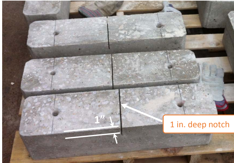
Figure 3.12 1 inch notch at mid-span of beams
