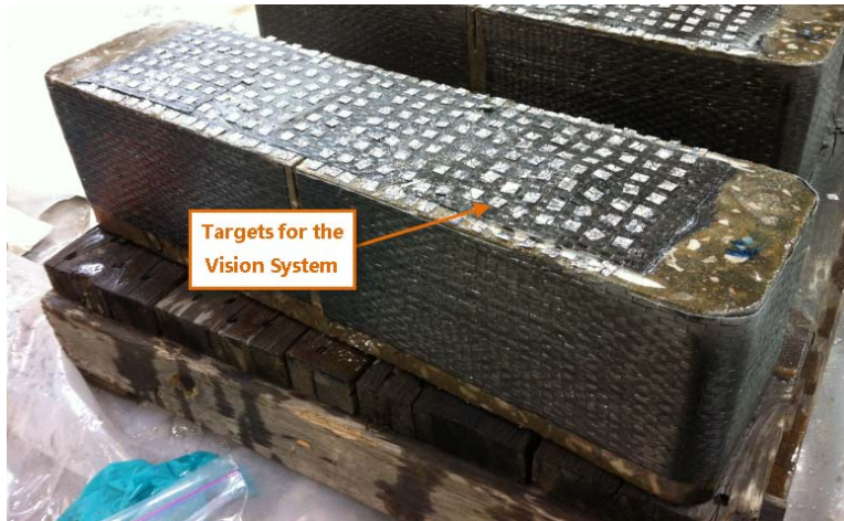
Figure 2.22 Targets used by the Vision System
