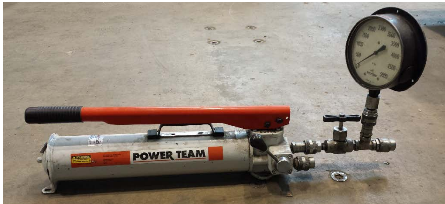
Figure 3.25 Hand pump used to load specimens
