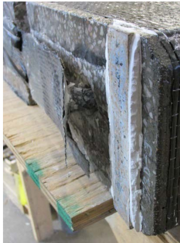
Figure 4.3 Specimen with anchor pull-out failure mode
