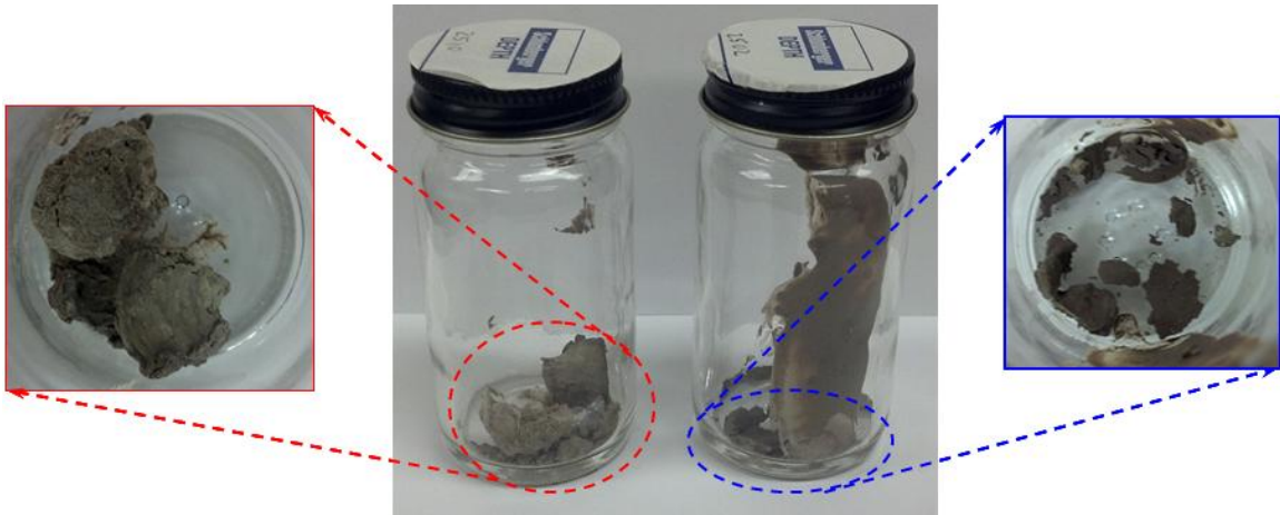
Figure 8.12: Core Plugs from the Field (broken apart and muddy looking).
