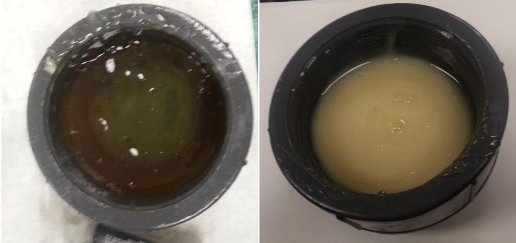
Figure A1.8: Epoxy and hardener before mixing (left) and after mixing (right).
