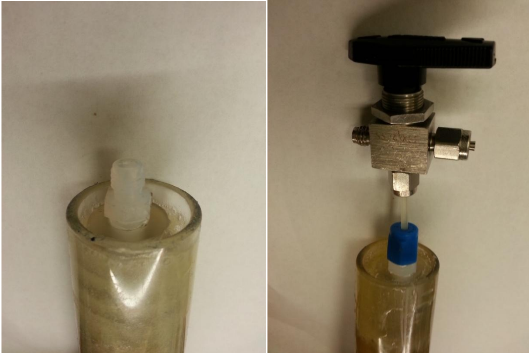
Figure A1.10: Core with NPT fittings attached to the endcap (left) and with Swagelok valve attached to the NPT fittings (right).
