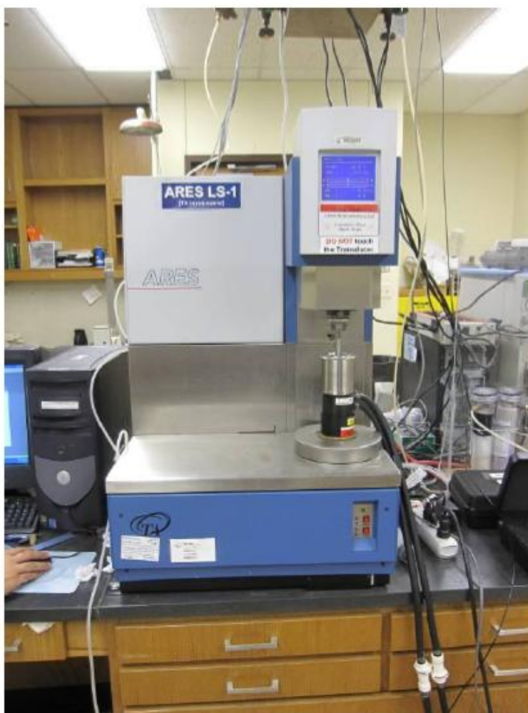
Figure A2.1: Picture of a rheology test using an ARES-LS1 rheometer (Lee, 2009).
