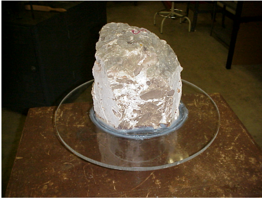
Figure 4.6 Rock sealed on a plastic disk, which has a hole in the center that allows water to flow through; the diameter of the hole is 23 cm.
